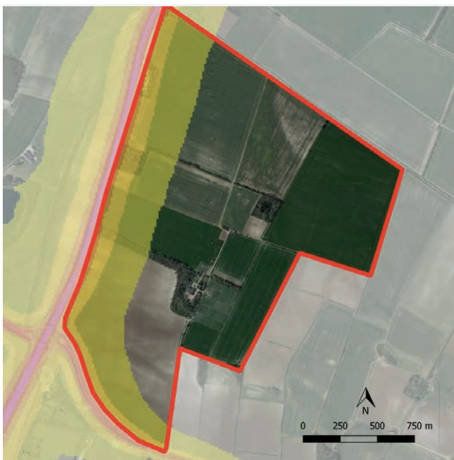
Site location with night time sound levels based on DfT traffic data
