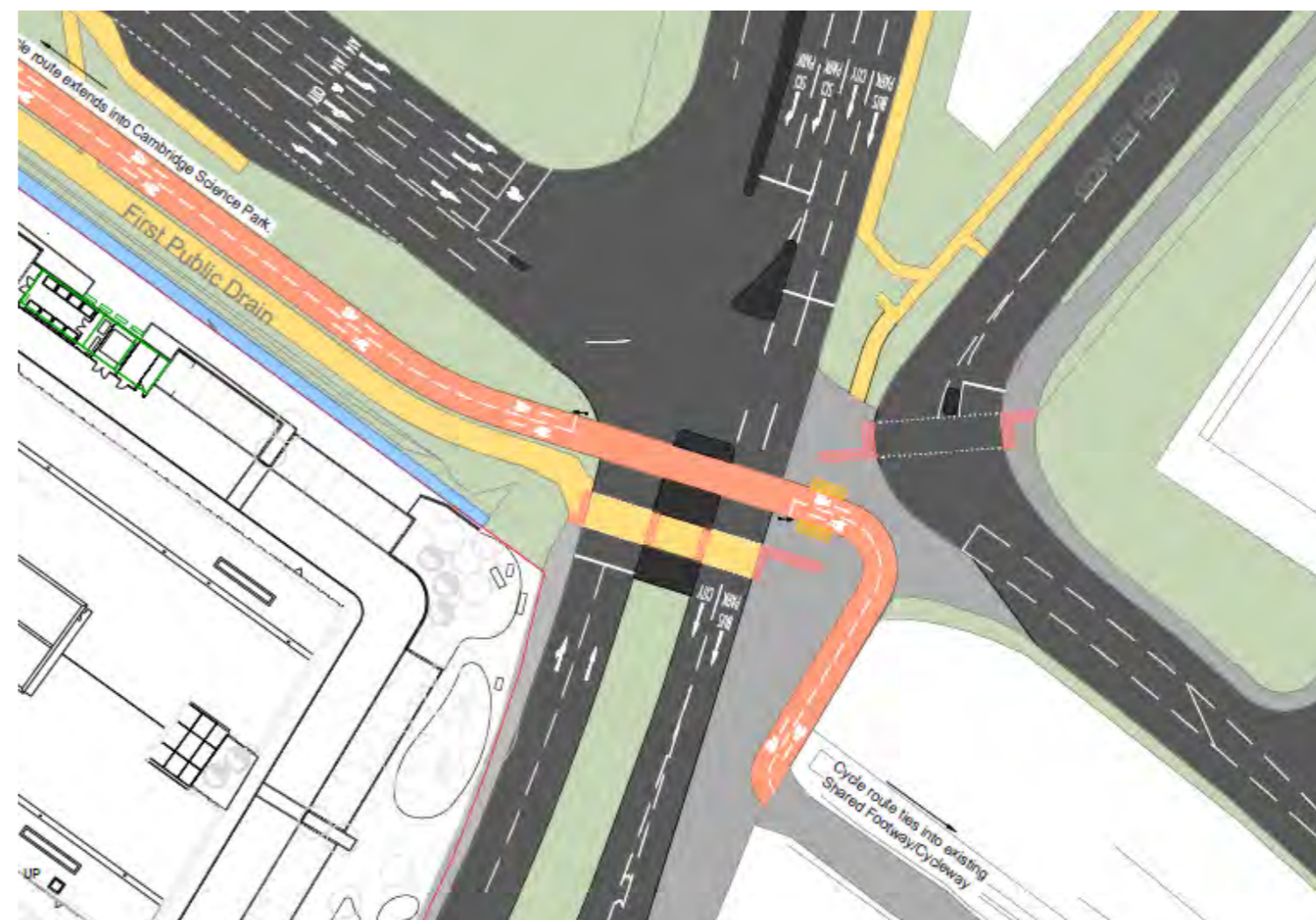
Improved Milton Road crossings can include at-grade, dedicated cycle crossings providing separate facilities for pedestrian and cyclists without being asked to divert to alternative structures such as underpasses or bridges.
