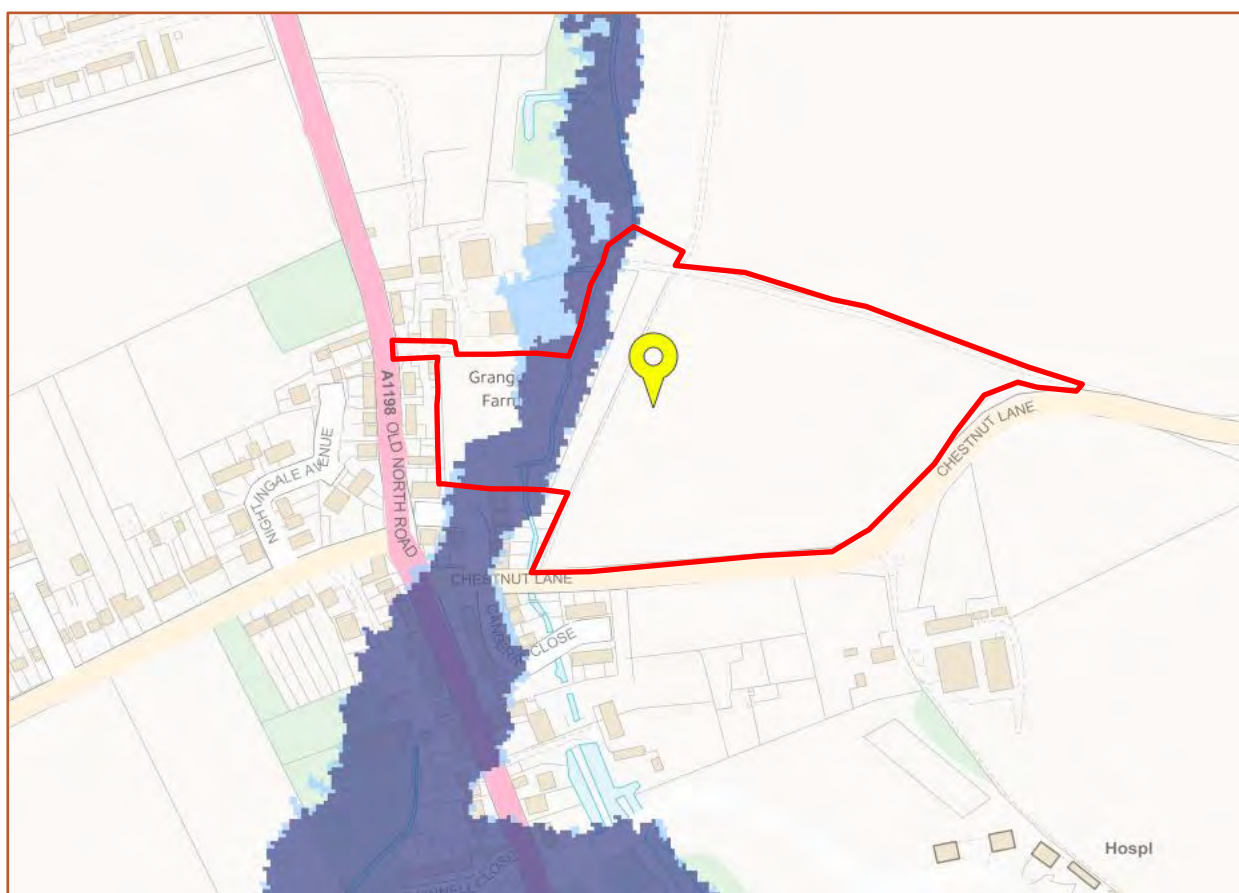
Figure 6: EA Flood Map for Planning extract, showing fluvial flood risk to the site
