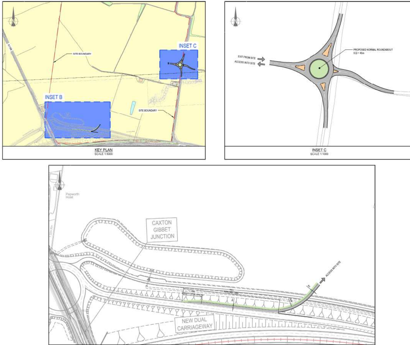
FIG 13 POTENTIAL VEHICULAR ACCESS ARRANGEMENTS VIA ROGUES LANE / BROCKLEY ROAD AND ENTRY ONLY ACCESS VIA THE A428 EASTBOUND ON-SLIP AT NEW CAXTON GIBBET JUNCTION
