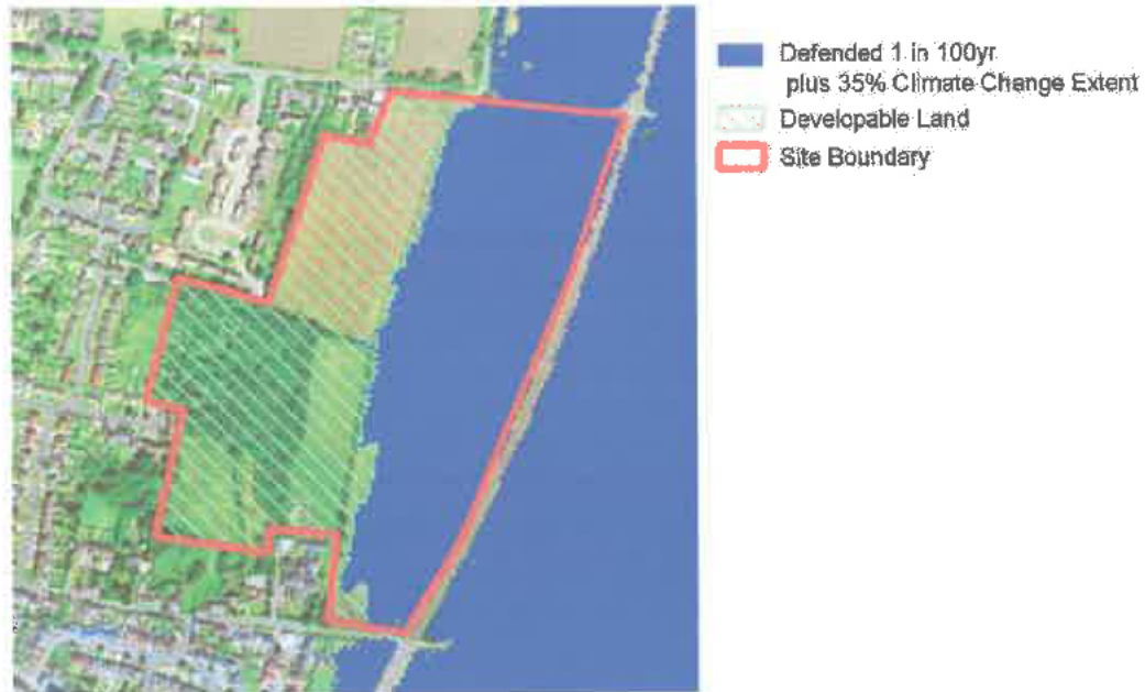
Figure 3-1 - 1 in 100 Year plus Climate Change Maximum Flood Extent in 'Defended' Scenario and Identified Potential Developable Land Area.
