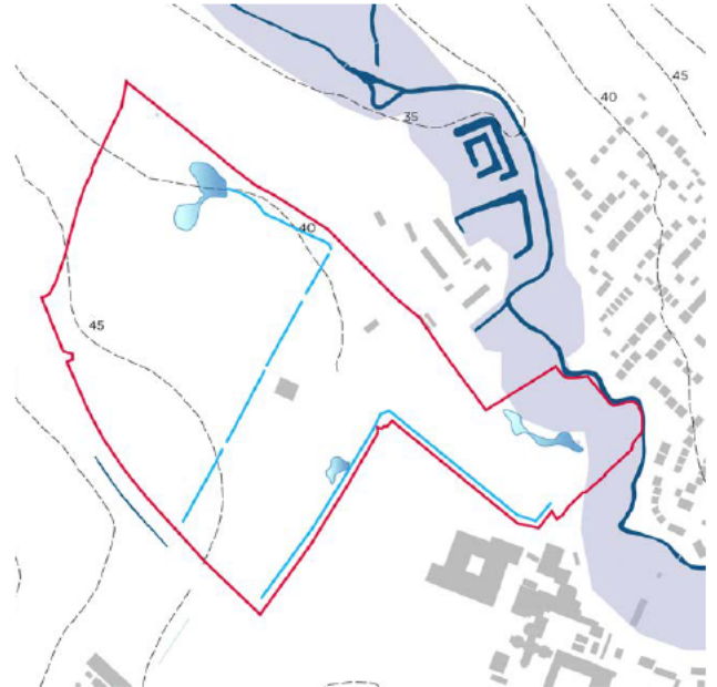
4. Sustainable Surface Water Drainage - SuDs strategy consisting of attenuation ponds, swales and permeable paving.
