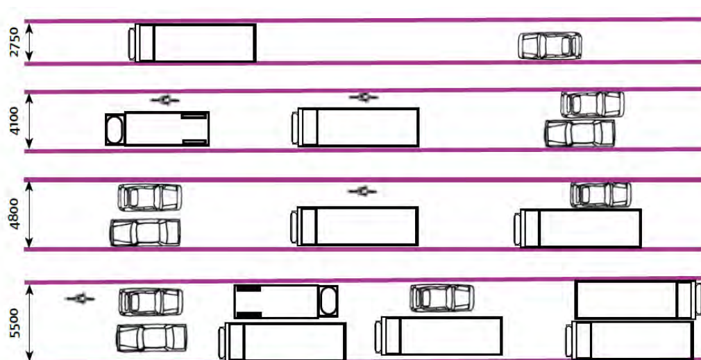
Figure 7.1 Illustrates what various carriageway widths can accommodate. They are not necessarily recommendations.
