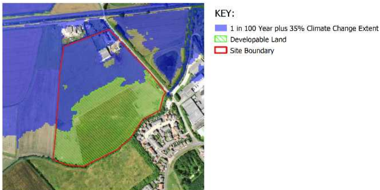
Figure 3-1 - 1 in 100 Year plus Climate Change Maximum Flood Extent in 'Defended' Scenario and Identified Potential Developable Land Area.
