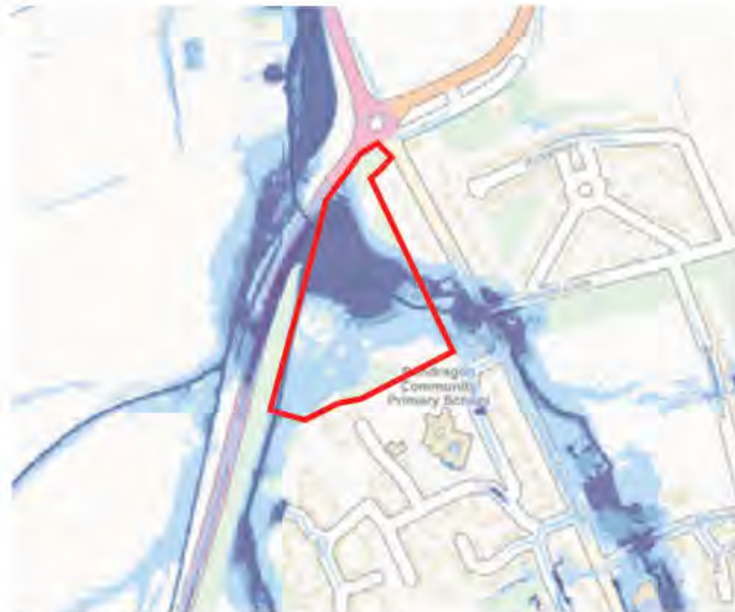
Figure 33; Surface water flood risk - Site B
