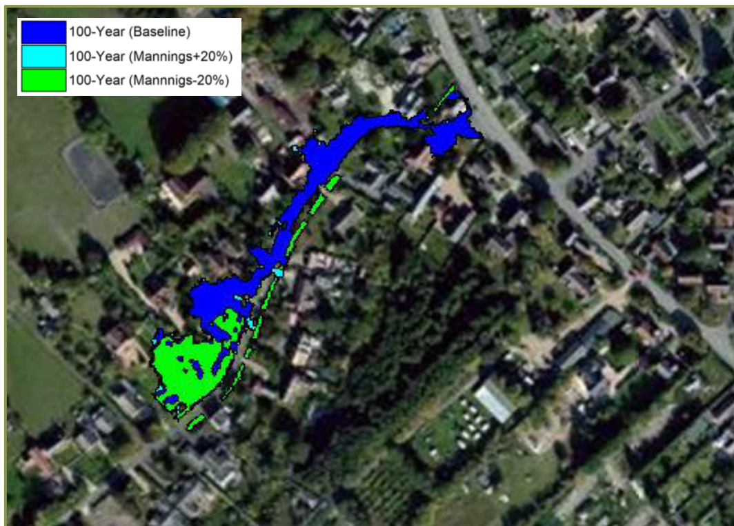
Top: Manning’s extent changes at the Site Bottom: Manning’s extent changes in Chiswick End
