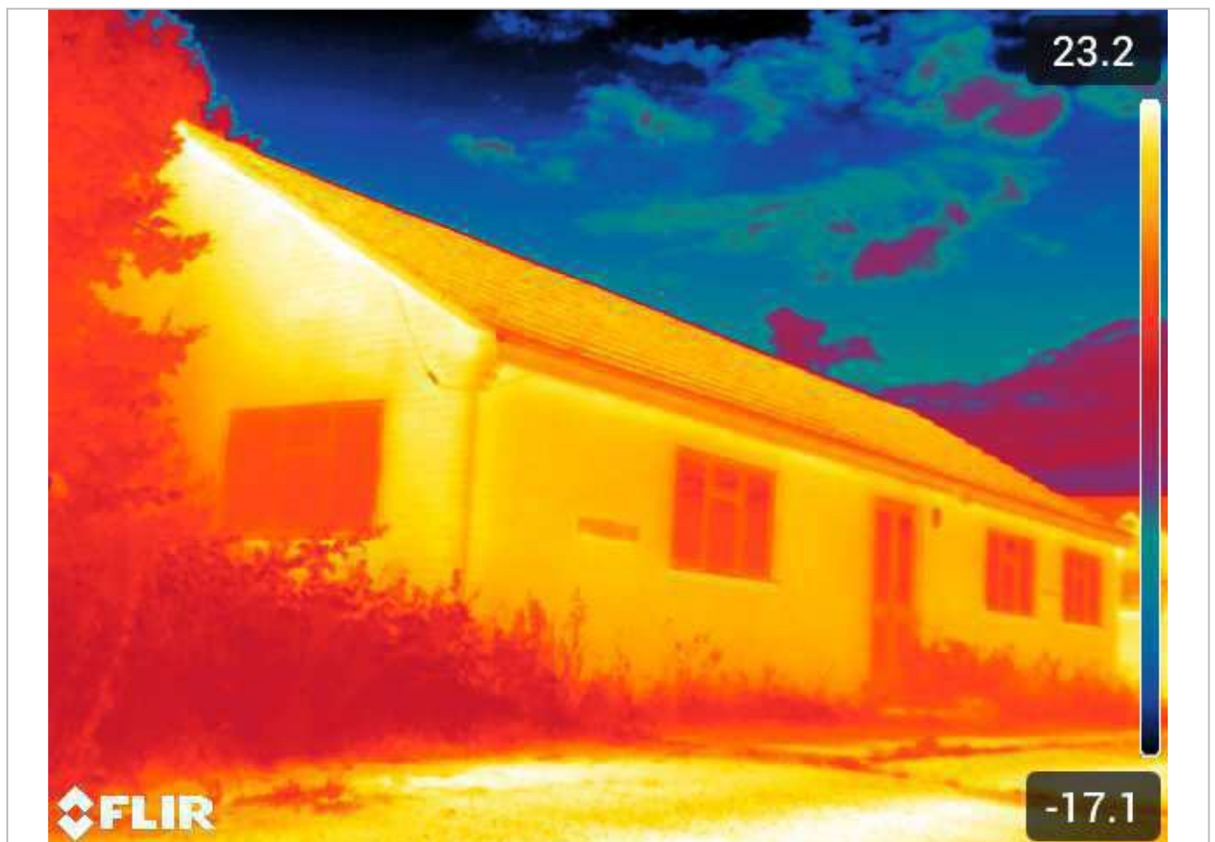
FLIR T540 (464 x 348 pixel resolution) with 42 degree lens = bat in flight detection distance of 51 m. Camera located 26 m from furthest point of building
