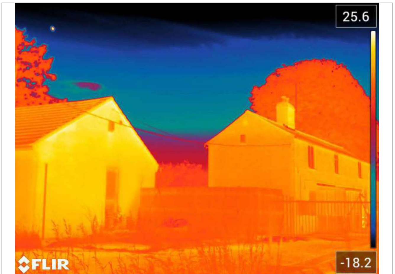
FLIR T1020 (1024 x 768 pixel resolution) with 45 degree lens = bat in flight detection distance of 104 m. Camera located 35 m from furthest point of building
