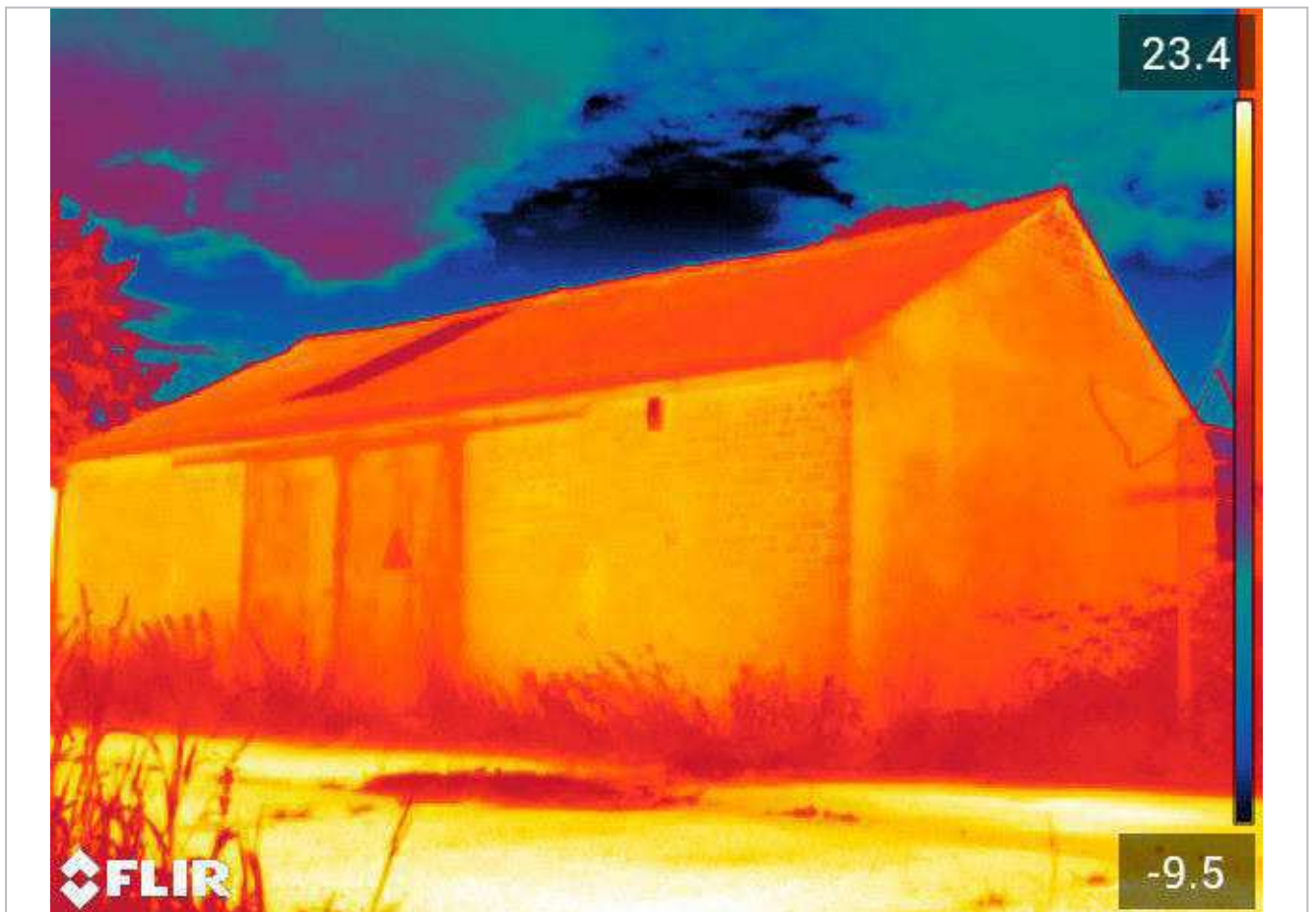
FLIR T860 (640 x 480 pixel resolution) with 42 degree lens = bat in flight detection distance of 66 m. Camera located 23 m from furthest point of building
