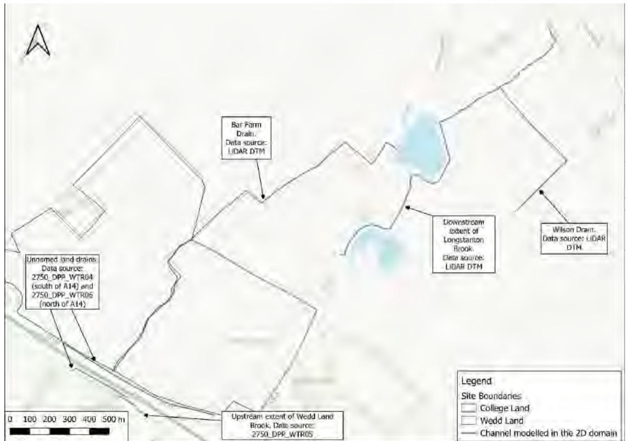
Figure 8: Channels modelled in the 2D domain and associated data sources.
