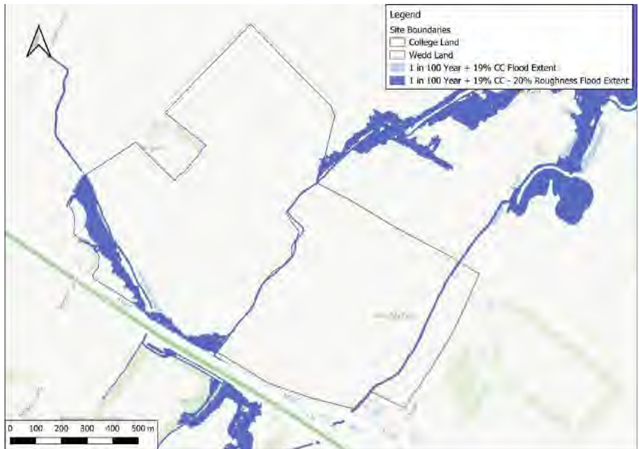
Figure 10: Flood Extent Comparison - 1 in 100 Year plus 19% Climate Change and 1 in 100 plus 19% Climate Change - 20% decrease in Manning's N roughness coefficient
