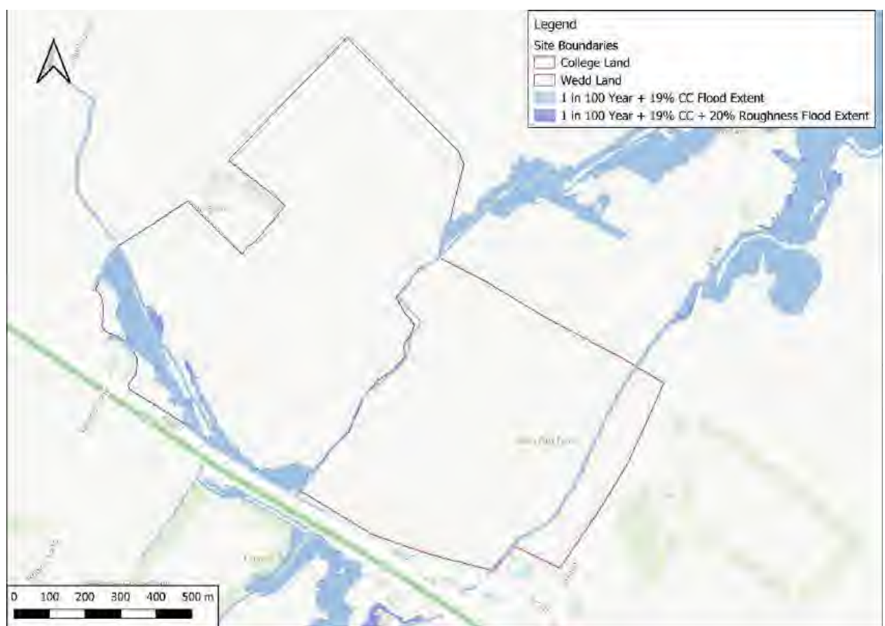
Figure 11: Flood Extent Comparison - 1 in 100 Year plus 19% Climate Change and 1 in 100 plus 19% Climate Change + 20% increase in Manning's N roughness coefficient
