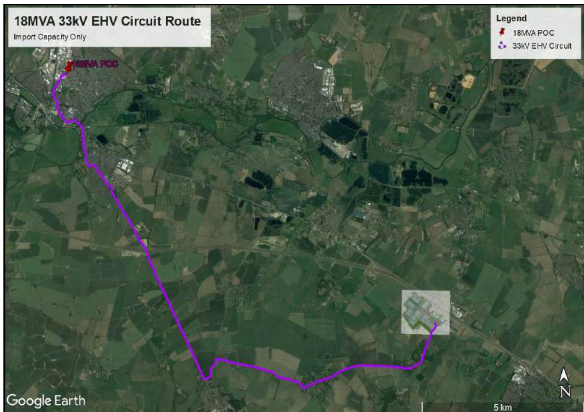
Figure 8.2.1– Anticipated 33kV EHV cable route from 18MVA POC to development area.
